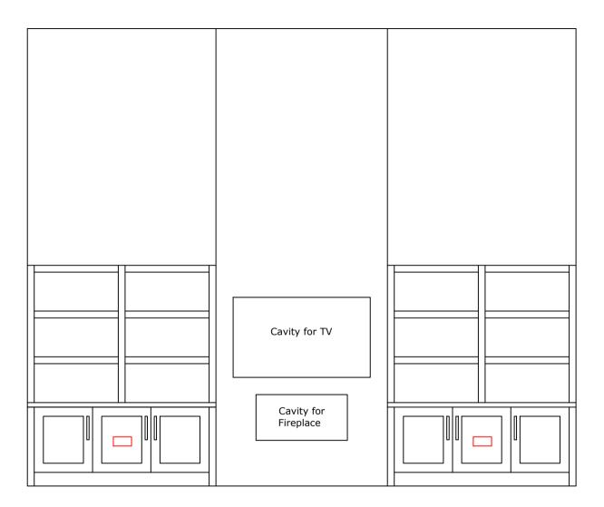
Elevations of TV Unit. Central section is a stud wall to is to be built. Power and whatever cables are needed for TV the be located behind TV section. Power may also be needed for Fire. Low sockets left and right behind TV unit for lighting in upper section where the open shelving is.
