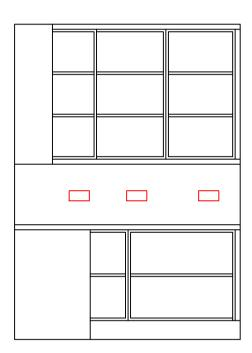
Elevations of walls in Pantry. Low socket for chest freezer. Isolator needed for this. Sockets as desired after that. High socket as shown or else trailing lead (preferable for under-counter lighting (if desired). However many sockets you think you might need after that.
