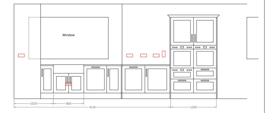
Keep plumbing pipes centered is sink section (800mm wide area shown). Also put dishwasher socket here. If other low sockets are required they can be put here (for kicker lights for example). Power for Ovens and warming drawer to be brought out to the area shown. Isolators needed for these can be on wall to left of Ovens. Isolator will also be needed for Hob, Extraction and any other power on Island. These can be put on this wall also, discuss with electrician.
