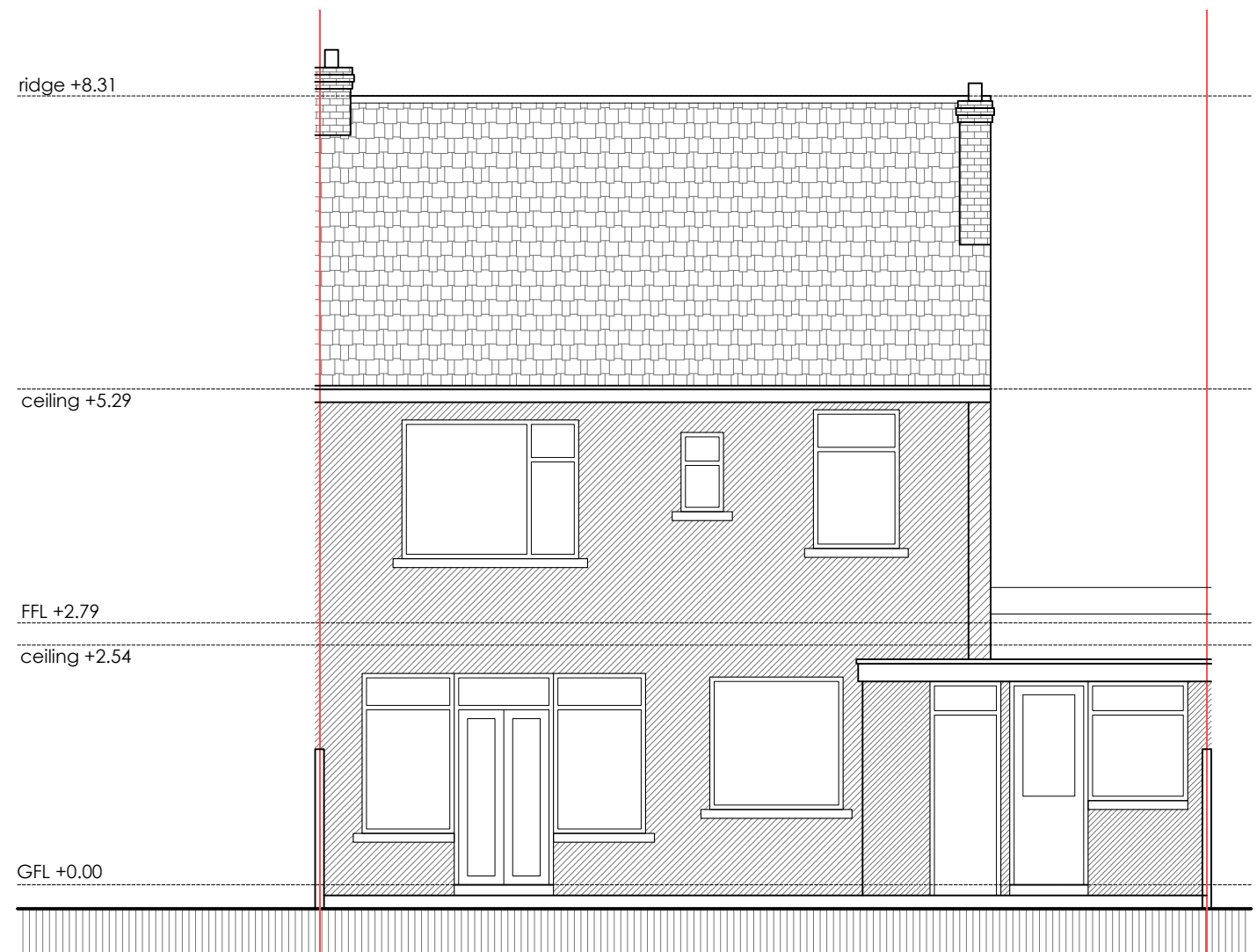
EXISTING REAR ELEVATION (N) scale 1:75 @ A3
