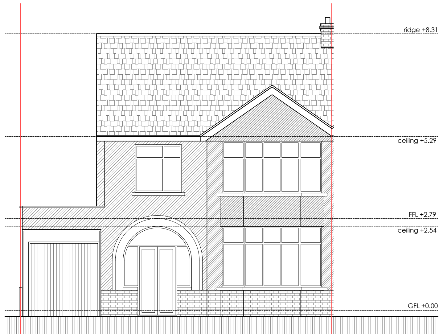
EXISTING FRONT ELEVATION (S) scale 1:75 @ A3
